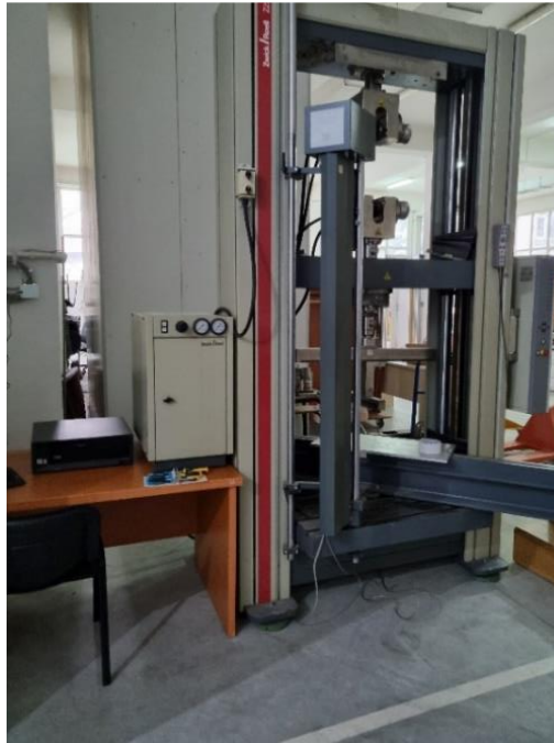
Figure 2 Zwick/Roell model SC-FR250SW.A4K.001
