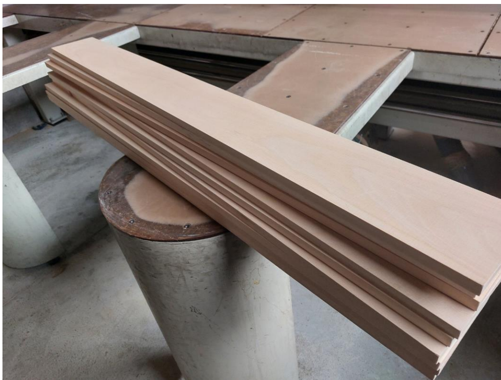
Figure 3. Prepared BEECH planks with a thickness of 15 mm
