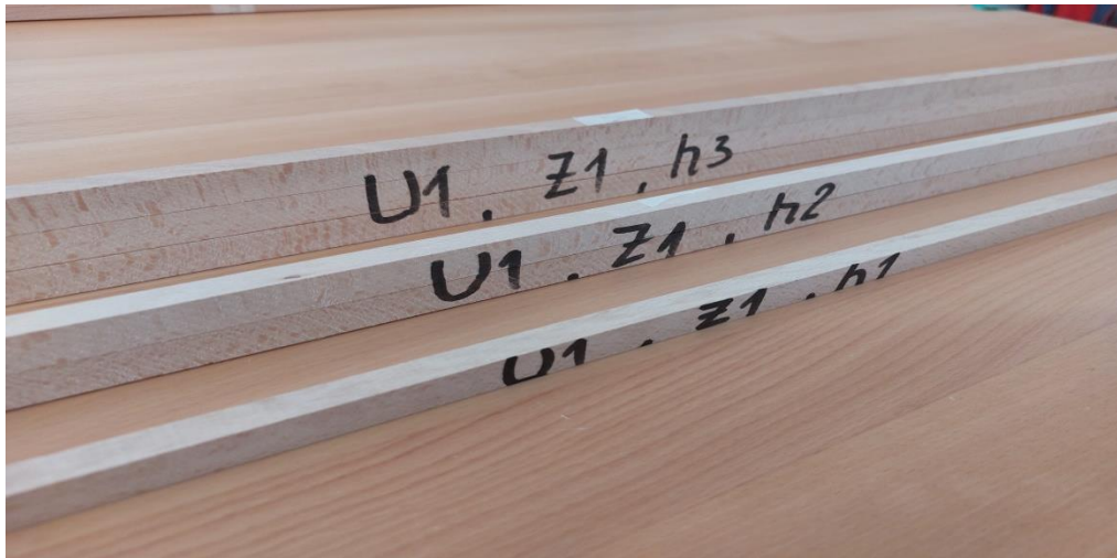
Figure 8. BEECH samples obtained at feed speed U_1=12 \text{mmin}^{-1} , number of teeth Z_1=40 , for cutting height h_1=15\text{mm} , h_2=30\text{mm} and h_3=45\text{mm}
