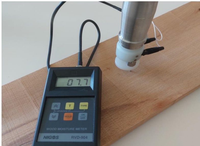
Figure 10. Moisture meter type NIGOS RVD-904
