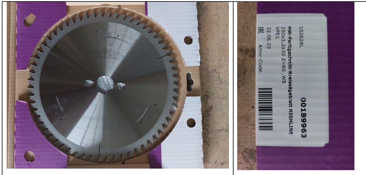
Figure 6. Circular saw with a diameter D=250\text{mm} , thickness 3.2\text{mm} and number of teeth Z_2=60
