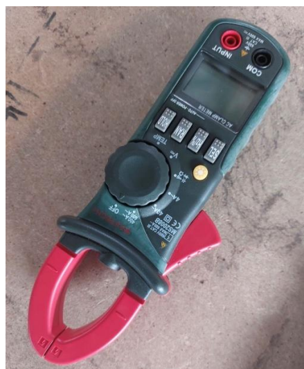
Figure 12. Voltage clamp MASTECH MS 2008B
